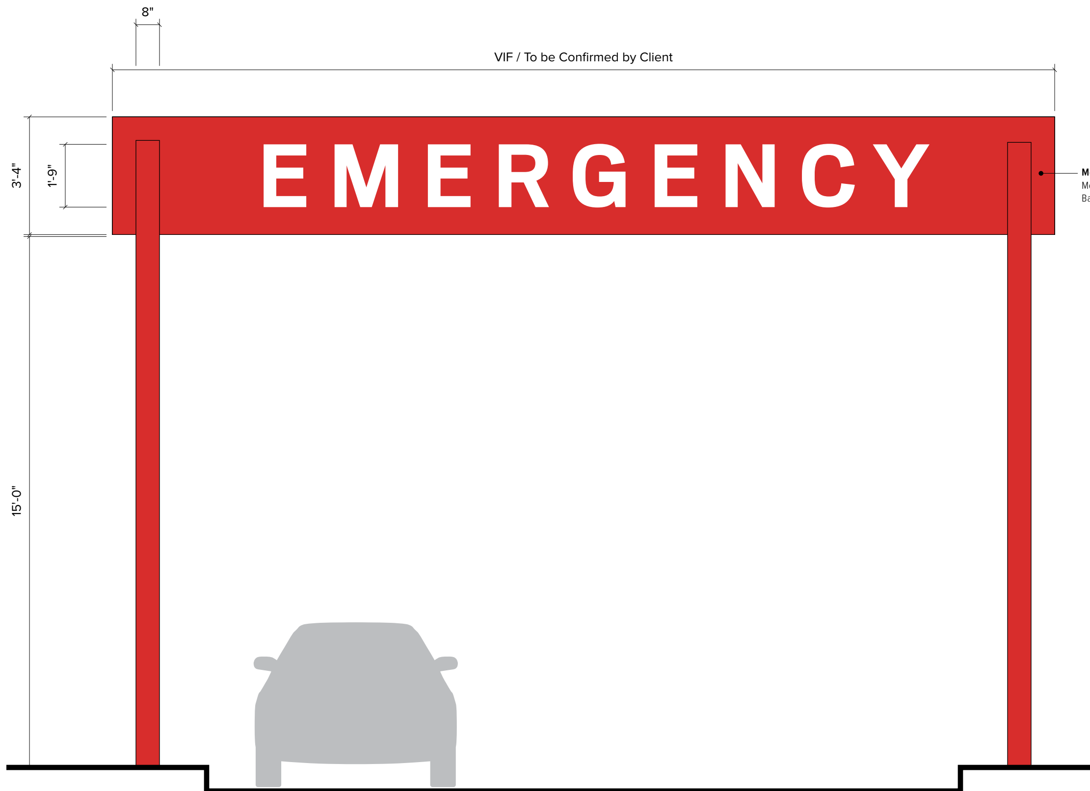
1 Installation Elevation - Sign Type R 3/8" = 1'-0"
