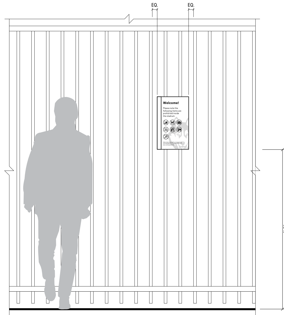
1 Installation Elevation - Sign Type Q2 3/4" = 1'-0"
